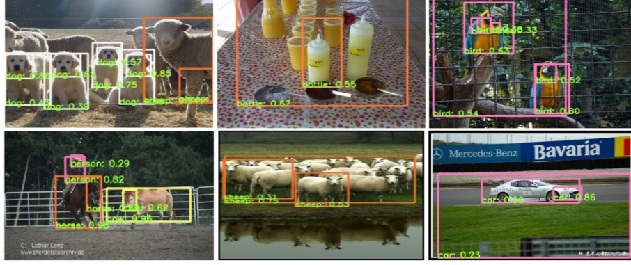
Fig. 2: Example of box-in-box (BiB) pairs among the predictions of the weakly-supervised object detector. The existence of such pairs is an indicator of the detector’s failure on those images. Best viewed in color.
