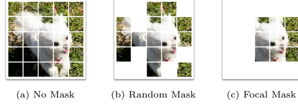
Fig. 3: Masking strategies. When applying a Random Mask, we randomly drop patches across a global view of the image. When applying a Focal Mask, we randomly select a local continuous block of an image, and mask everything around it. We typically leverage both Random and Focal Masking strategies when pre-training with MSNs.
