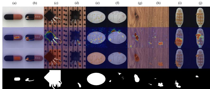
Fig. 7: DSR localization examples on the MVTec dataset. From top to bottom, the input image, the overlay of the DSR segmentation output, the overlay of the ground truth mask and the ground truth mask are shown.
