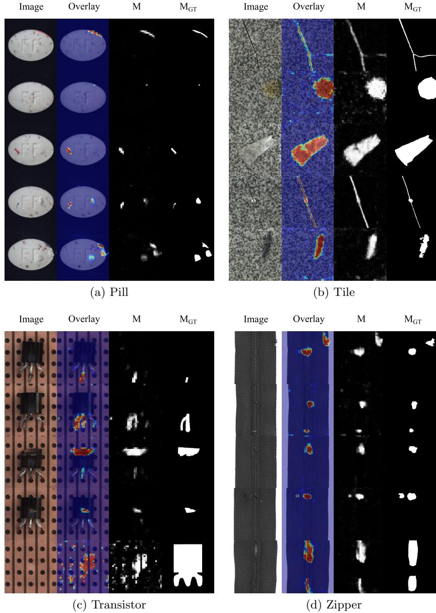
Fig. 4: Qualitative examples on the MVTec dataset [1]. The input image, overlaid DSR output map, DSR output map and the ground truth map are shown from left to right.
