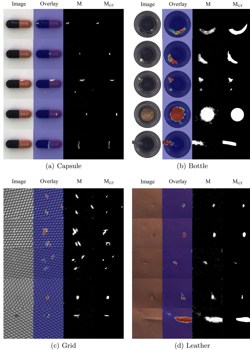
Fig. 3: Qualitative examples on the MVTec dataset [1]. The input image, overlaid DSR output map, DSR output map and the ground truth map are shown from left to right.
