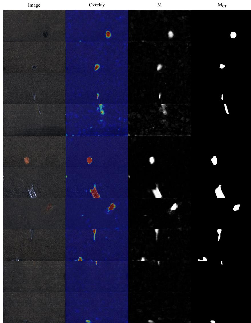
Fig. 2: Qualitative examples on the KSDD2 dataset [3]. The input image, overlaid DSR output map, DSR output map and the ground truth map are shown from left to right.
