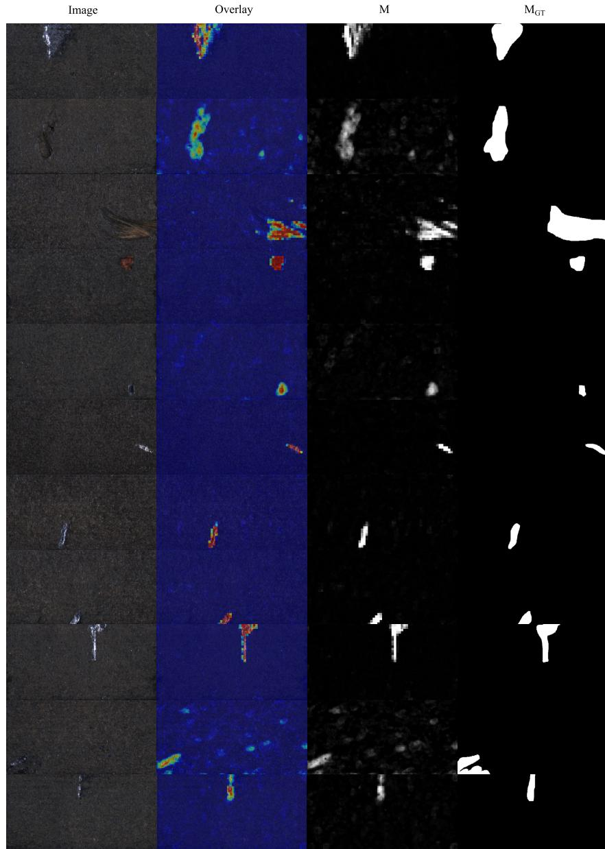
Fig. 1: Qualitative examples on the KSDD2 dataset [3]. The input image, overlaid DSR output map, DSR output map and the ground truth map are shown from left to right.
