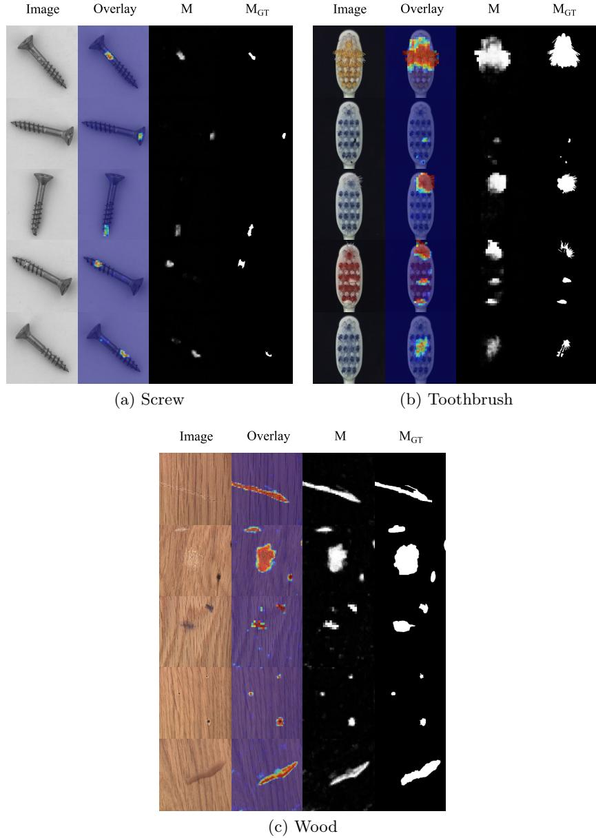
Fig. 6: Qualitative examples on the MVTec dataset [1]. The input image, overlaid DSR output map, DSR output map and the ground truth map are shown from left to right.
