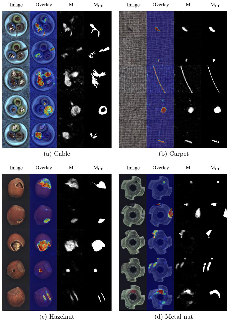
Fig. 5: Qualitative examples on the MVTec dataset [1]. The input image, overlaid DSR output map, DSR output map and the ground truth map are shown from left to right.
