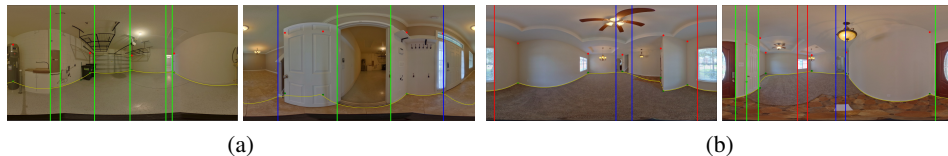
Fig. 4: Mistakes made by the joint HorizonNet + W/D/O model. Vertical lines indicate start and end columns for each W/D/O object – w indow, d oor, and o pening. The yellow contour indicates the predicted floor-wall boundary, and dots indicate corner predictions (floor-wall corners in green, and ceiling-wall corners in red). Left and right images are panoramas across which we seek to match W/D/O objects. Top: A circuit breaker panel is mistakenly identified as a door ( top left ), but redundancy still allows matching of the true garage door. This allows a relative pose hypothesis to be generated between the foyer and garage panoramas, that have very little visual overlap. Bottom: A false negative window prediction and inaccurate opening prediction ( bottom left ) makes matching with the ( bottom right ) panorama impossible using W/D/O.
