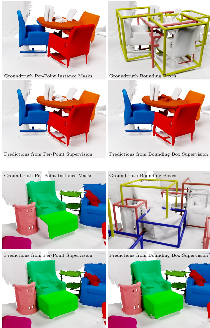
Fig. 4: Qualitative Instance Segmentation Results on ScanNet [3] Individual instance masks are colored randomly and match the ground truth instance mask colors. Left: results from full per-point supervision. Right: weak bounding-box supervision.
