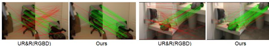
**Fig. 3.** Visualization of pairwise matching results by UR&R (RGB-D) [15] and our method (trained on the 3D Match dataset [39]). We show the positive correspondence (*i.e.*, the matching error  $< 10\text{cm}$ ) and the negative correspondence (*i.e.*, the matching error  $\geq 10\text{cm}$ ) as the green lines and the red lines, respectively. Best viewed on screen.
