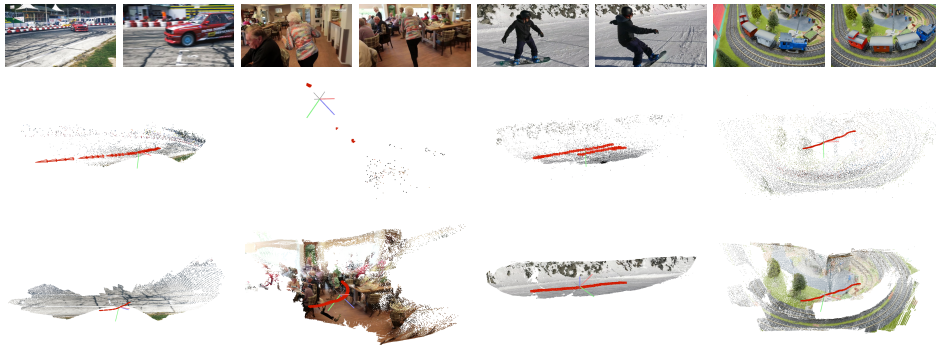
Fig. 6. Top row: COLMAP [61]. Bottom row: Ours. Qualitative comparison on in-the-wild videos from DAVIS [52]. Our dense indirect system produces robust camera trajectory and denser maps for videos with complex foreground motion
