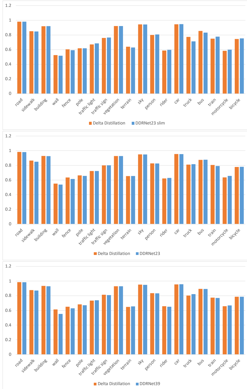
Fig. 1: Per class IoU on Cityscapes for different DDRNet models. Note that Delta distillation does not exploit any single class, but rather improves upon several or retains overall IoU at a lower cost.
