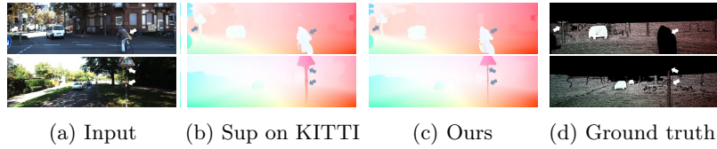
Fig. 5: Qualitative results on KITTI. We visualize optical flow predicted by (b) supervised on target dataset and (c) semi-supervised w/o target label. Note that sparse ground-truth (d) is not sufficient to make a clear boundary of objects (marked with arrows), while our method shows better results
