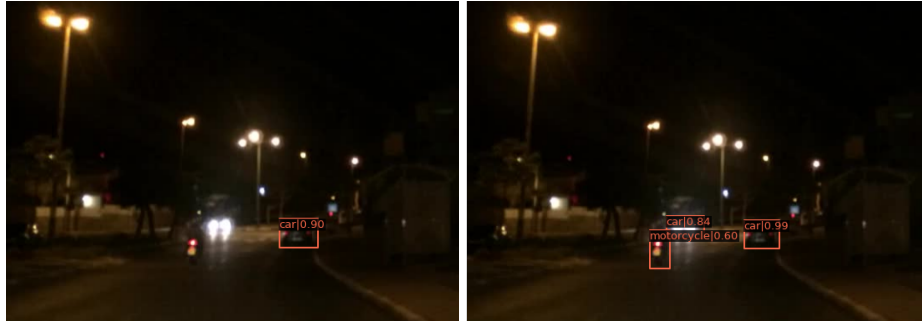
Fig. 10: A false negative motorcycle at night on the road (left) fixed to a true positive detection (right) using TALISMAN.
