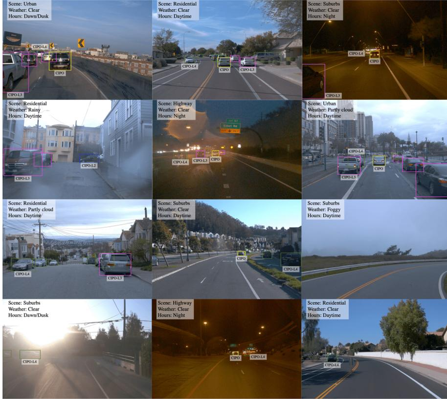
**Fig. 6.** Visualization example of CIPO and Scene tags annotation in OpenLane dataset
