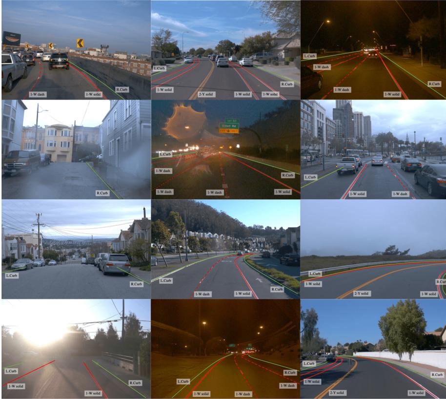
Fig. 5. Visualization example of lane annotation in OpenLane dataset
