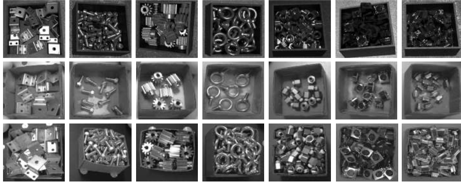
Fig. 1. Seven object models provided by ROBI [11]. Zigzag, Din Connector, and D-Sub Connector are three asymmetric objects, and the remains are symmetric objects. Din Connector and D-Sub Connector are composed of two different materials.
