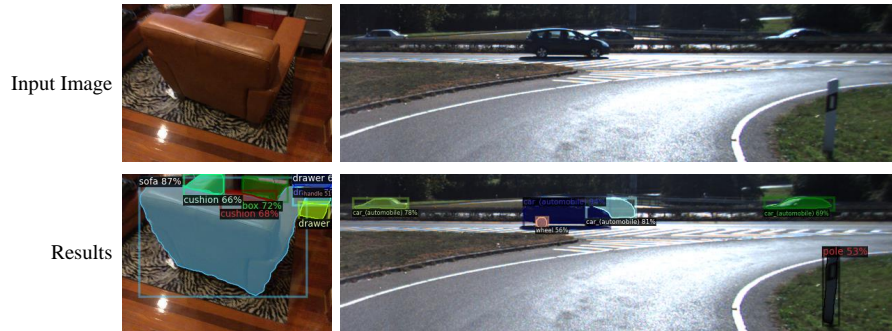
Fig. 2: Examples of the segmentation results output by GroundedSAM [7]. The images are from the ScanNet [2] (left) and SemanticKITTI [1] (right) datasets.
