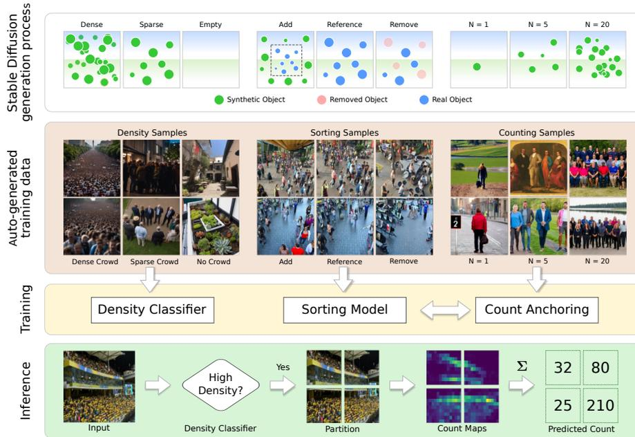
**Fig. 3: Workflow.** Our framework uses simple prompts to create synthetic data for training a sorting model, a density classifier, and a count anchoring network. These elements are combined into a model which can accurately count diverse object categories even within dense images by subdividing them into smaller, more manageable areas.
