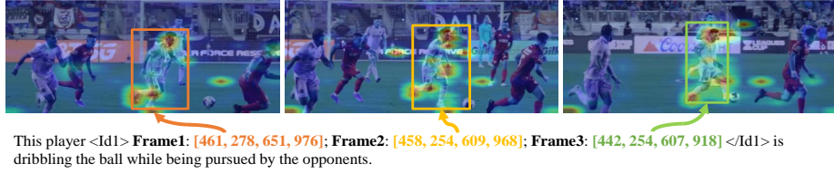
Fig. 5: Attention map visualization. To facilitate the observation, we map the attention between the box responses and the visual tokens of each frame for visualization.
