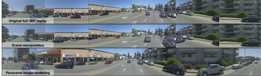
Fig. 8: Realistic and controllable multi-camera simulation on PandaSet. G3R reconstructs a manipulable 3D scene representation.
