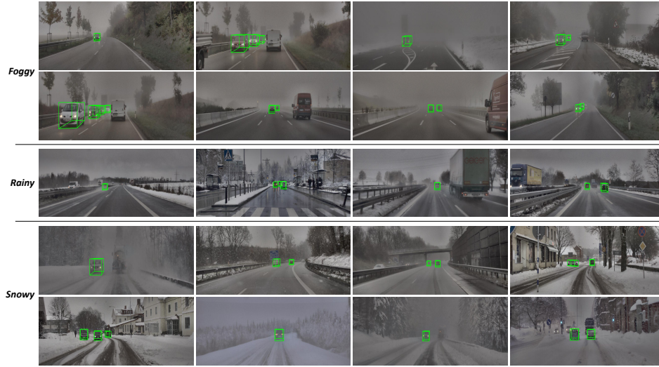
Fig. 6: 3D detection results on real-world images of various weather conditions.
