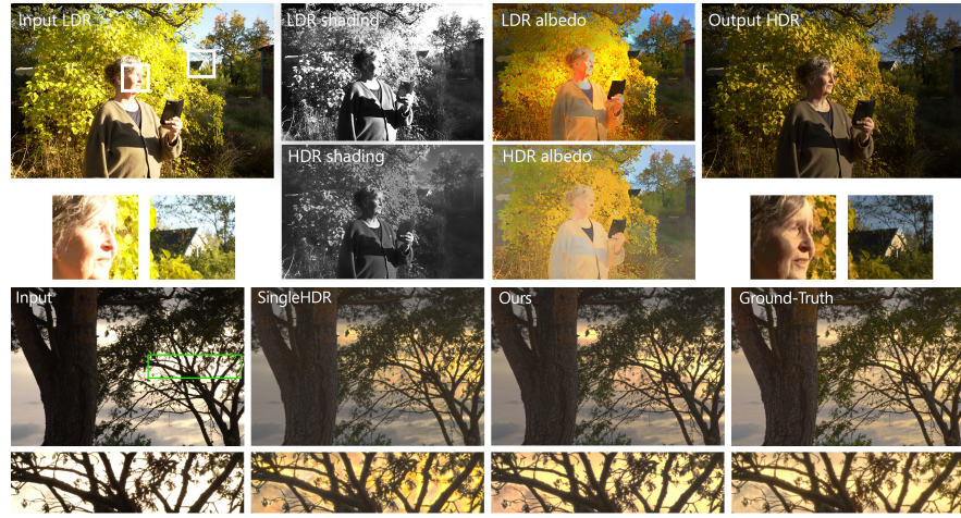
Fig. 1: In this work, we propose a physically-inspired HDR reconstruction pipeline by conducting reconstruction individually on intrinsic components. Our final reconstruction, as a result, is effective in recovering the high-luminance details and the lost colors.
