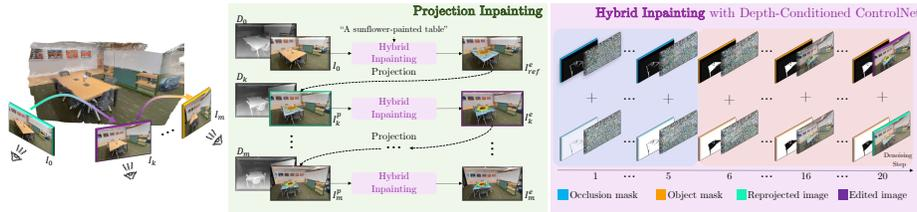
**Fig. 2: Overview.** Our input is a NeRF (with its posed input images) and per-view editing masks and an edit text prompt. We use the NeRF depth to condition the masked region inpainting. We reproject this edited result to a subsequent viewpoint and using a hybrid inpainting scheme that first only inpaints disoccluded regions and then refines the entire masked region. This is done by changing the inpainting masks (indicated by the blue and orange blocks on the right side) during diffusion.
