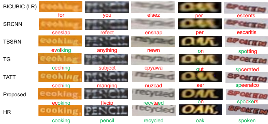
Fig. A.2: High resolution images generation by various state-of-the-art methods and the proposed method, failure cases for the proposed method. BICUBIC (LR) and HR indicate the input to the methods and ground truth, respectively. The text recognition results by ASTER [33] are shown under the images. The characters in green and red indicate correct and incorrect recognition results, respectively.
