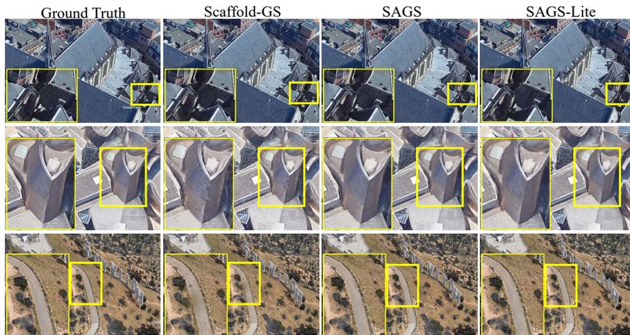
**Fig. 1: Depth Structural Preservation.** Comparison between the proposed and the Scaffold-GS method on the BungeeNeRF dataset. The proposed method can accurately capture sharp edges and high frequency details that Scaffold-GS method fails to model.
