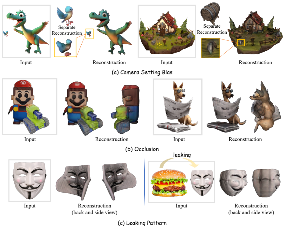
Fig. S2: “Multi-object gap” of models trained on Objaverse. (a) Camera Setting Bias. The reconstruction quality for small and non-centered objects will significantly downgrade compared to separate reconstruction. (b) Occlusion. The reconstruction results tend to blend when an object is occluded by another. (c) Leaking Pattern. The shape and texture of an object will be influenced by other objects in the input image.
