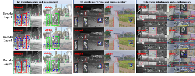
Fig. 5: Visualization of feature sampling at different semantic levels in different decoder layers. Different colors of points represent the results of sampling in different semantic layers, where blue, green, and red represent sampling points on low-level, middle-level, and high-level semantic features maps respectively. Brightly colored and large points indicate relatively high attention weights. (a) The green boxes in the visible image represent aligned bounding boxes, which show the sampling points in each modality are concentrated on the right instance locations. (b) Objects occluded by background and smoke tend to predominantly focus on the infrared modality at subsequent decoder layers. (c) Objects in good illumination conditions and those less distinguishable in the infrared modality tend to predominantly focus on the visible modality at subsequent decoder layers.
