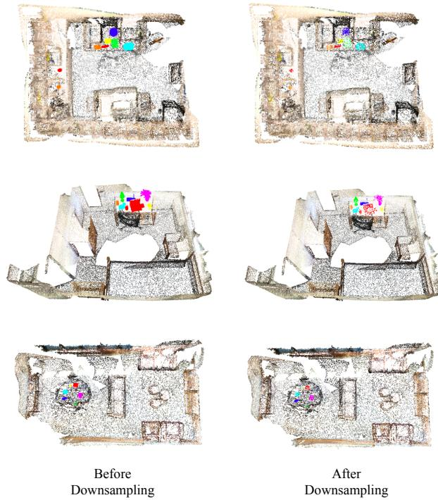
**Fig. 3:** Visualization of scenes in TO-SCENE before (originally provided in [1]) and after (our TO-SCENE-down benchmark) downsampling. After downsampling, the density of points on small objects is closer to others, which is more realistic.
