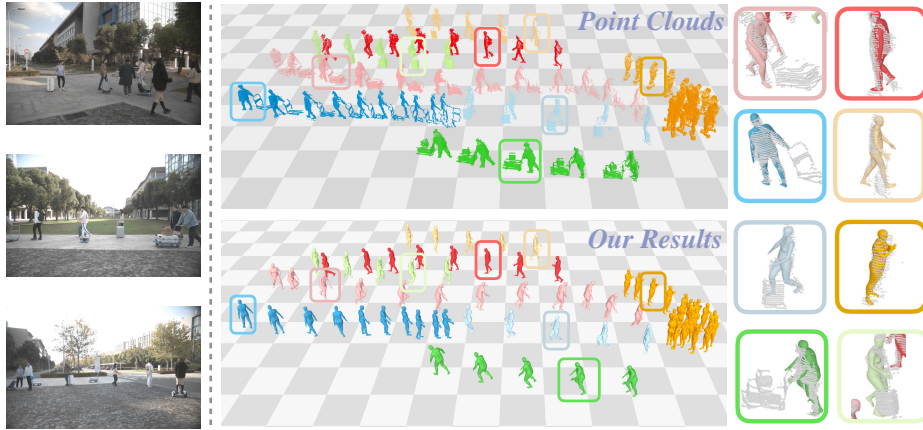
Fig. 1: Visualization of the motion capture performance of LiveHPS++ in a real-time captured scenario with complex human-object interaction. The left exhibits images for reference, the middle shows the noised point clouds (top) and our corresponding mesh model results (bottom). We zoom in some cases on the right for clearer demonstration, where point clouds are drawn in white.
