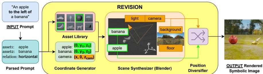
**Fig. 2:** REVISION parses a prompt into assets (objects) and the spatial relationship between them and synthesizes a symbolic image in Blender, placing the respective object assets at coordinates corresponding to the parsed spatial relationship.
