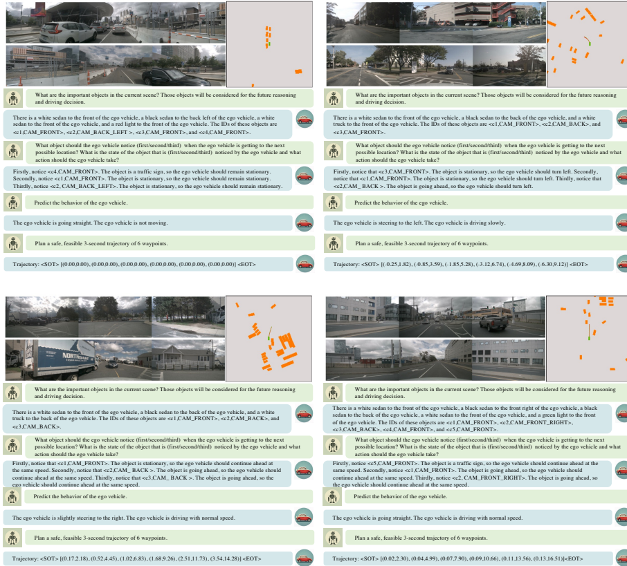
Fig. 1: Examples of the logical reasoning and trajectory planning of RDA-Driver. The planned trajectory and gt trajectory are in green and red respectively.
