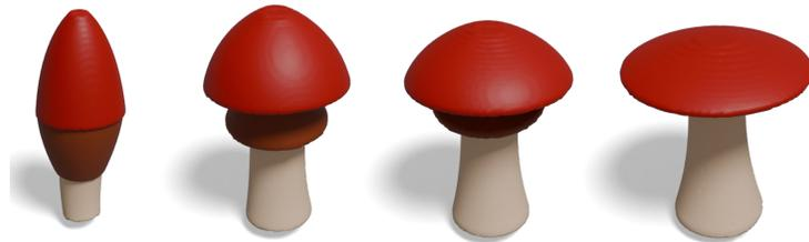
**Fig. 5:** A light bulb model is transformed into a mushroom by manipulating sweeping axis length, adjusting the scaling function, and enlarging the profile size. Each shape is represented by three primitives, with three control points each, employing a quadratic scaling function. In total, this representation requires 42 floating-point numbers.
