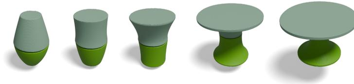
**Fig. 7:** A vase model transforms to a table by adjusting the sweeping axis length, and scaling function coefficients. Each shape is represented by two primitives, each with three control points and a quadratic scaling function, requiring a total of 28 floating-point numbers.
