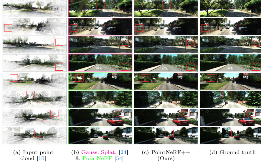
Fig. 4: Examples on KITTI-360 – We show novel-view renderings obtained with our method, 3D Gaussian splatting [24] (pink colored, 1-4 rows) and PointNeRF [54] (green colored, 4-8 row) on a challenging outdoors dataset, using the same point clouds as input. Our approach provides significantly sharper renderings with more details, and better coverage in areas without points, where Gaussian Splatting and PointNeRF produce highly salient artifacts highlighted with red boxes.
