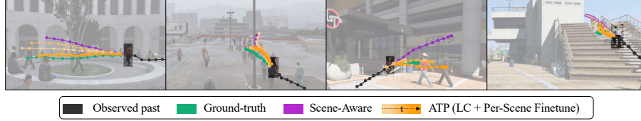
Fig. 4: Qualitative results over time. Our method’s predictions trained on a short number of human seconds (2%) are shown in light orange, to dark orange for a human seconds training time of 80%. With the latent corridor trained on a tiny amount of data, the predictions can significantly improve, but at times are close to the baseline. When more human seconds of data are seen, the adaptation results consistently improve.
