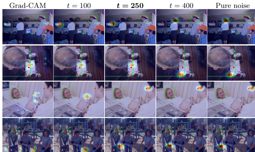
Fig. 5: Diffusion model output for noise added at different timesteps. Red dots represent the ground truth annotation. Adding noise at earlier steps generates outputs on high Grad-CAM response regions. Adding noise at later steps generates outputs similar to sampling from pure noise. Noise at step 250 is the best trade-off.
