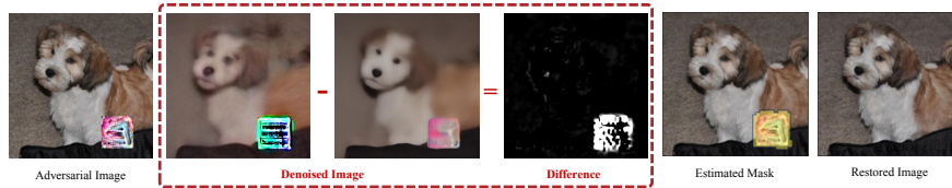
Fig. 1: The intriguing phenomenon of the diffusion model. A diffusion model is performed multiple times on the given adversarial image, and the differences between any two denoised images are pronounced within the adversarial patch regions, which can be leveraged to further pinpoint the location of adversarial patches.
