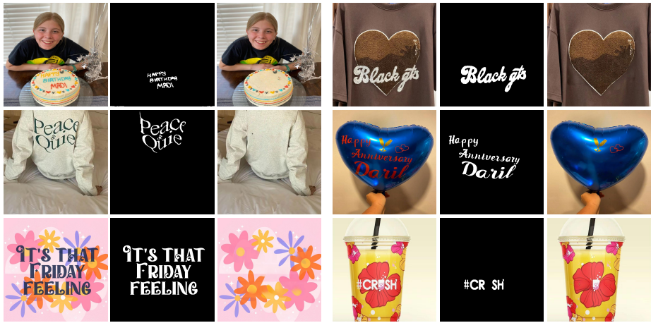
Fig. 2: Text removal visualization using predicted text masks from our WASNet and inpainting model LaMa [4]. Each sample includes the original image, the predicted mask, and the text removal result from left to right.
