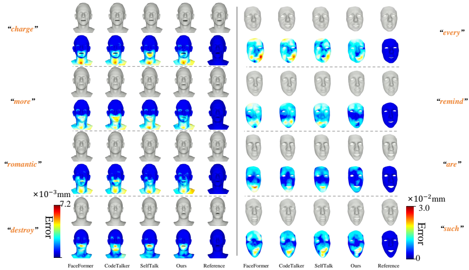
Fig. 2: Qualitative comparisons on VOCASET (left) and BIWI (right). We provide visual comparisons of facial animations synchronized with eight syllables extracted from the test speech sequences. The 1st, 3rd, 5th, and 7th rows display synthesized meshes and their corresponding ground-truths, while the 2nd, 4th, 6th, and 8th rows visualize the L2 loss for individual frames. Our method demonstrates more precise mouth movement and generates more natural and synchronized motion sequences visually.
