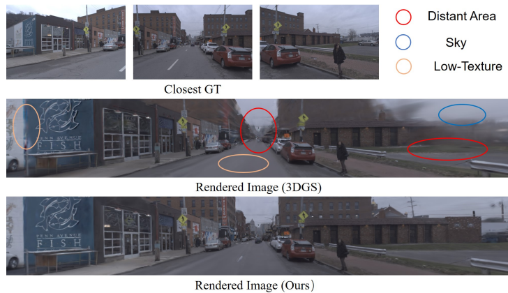
Fig. 1: Illustration of 3D Gaussian Splatting (3DGS) [22] and HO-Gaussian (Ours). Compared with 3DGS initialized by SfM points, our method has richer Gaussian geometric information in low-texture, sky and distant areas, and shows significant improvement in the task of synthesizing novel views.
