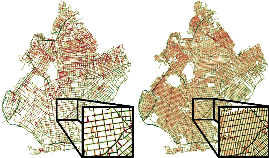
Fig. 1: We propose a method for image-driven traffic modeling, which can be used to create dense city-scale traffic models. (left) Historical ground-truth traffic data is often sparse as not all roads are traversed at all times. For example in Brooklyn on Monday at 8am, many roads are missing empirical speed data. (right) Our method can create a dense model of traffic flow at the same time.
