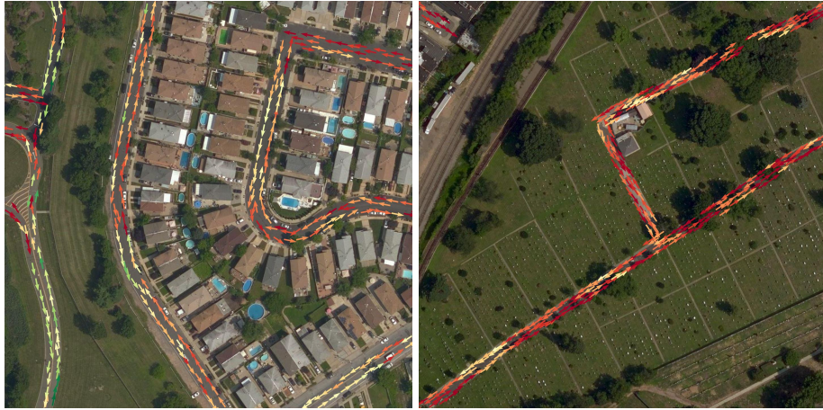
Fig. 7: The output of our approach on unseen locations visualized as a local motion model. We sample from locations predicted as road and visualize corresponding orientation estimates as vectors, colored by the predicted speed. Green (red) corresponds to fast (slow) traffic speeds.
