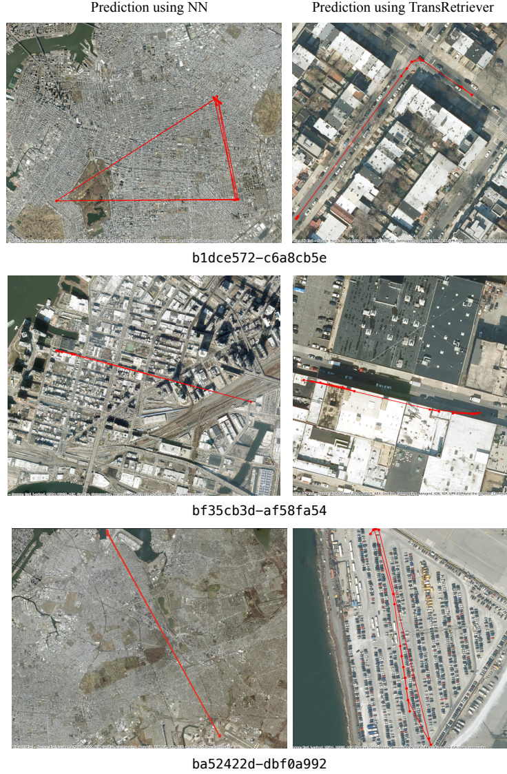
Fig. 4: Example trajectories obtained using our method when we use top-5 large aerial images in Sequence-to-Image inference. The first column depicts trajectories utilizing nearest neighbor (NN) retrieval, and the second column employs our TransRetriever module. Note that the aerial images shown here don't all have the same Ground Sampling Distance due to the NN predictions being way off from each other. Our proposed TransRetriever module significantly stabilizes the trajectories, yielding temporally consistent output.
