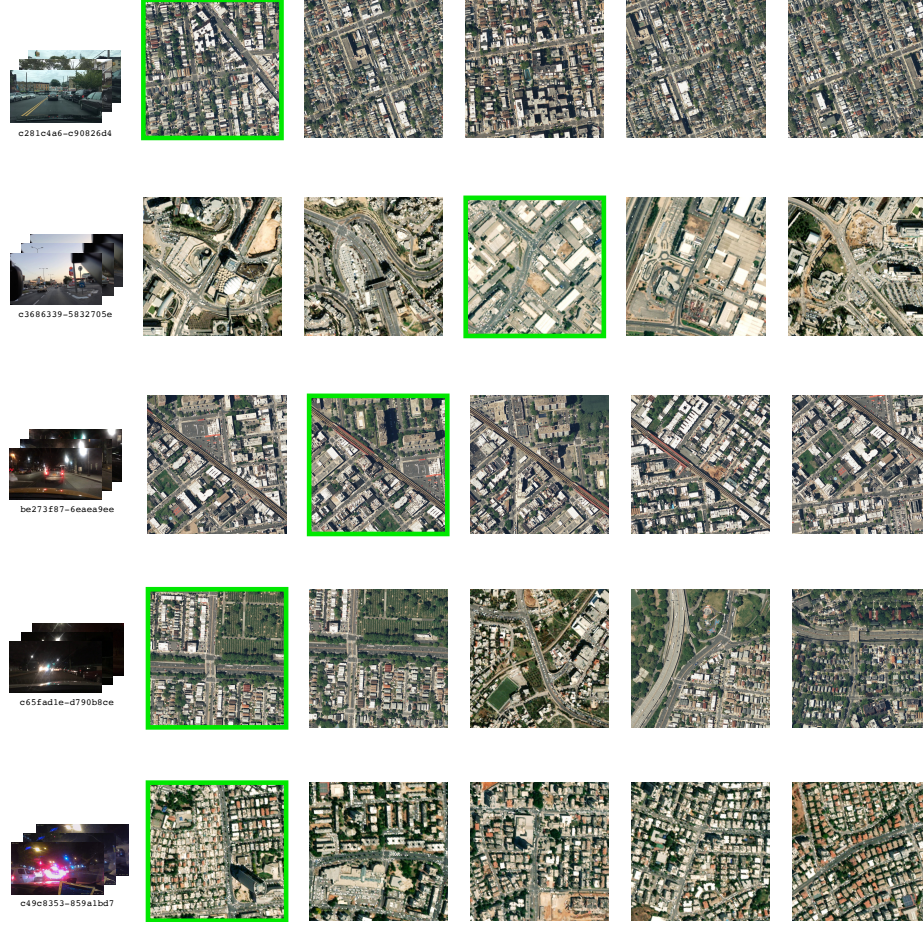
Fig. 2: Top-5 large aerial images retrieved using our method for a given street-view video. The green outline indicates correct predictions. For effective comparison in future works, we have provided the video-id for each sample we present here.
