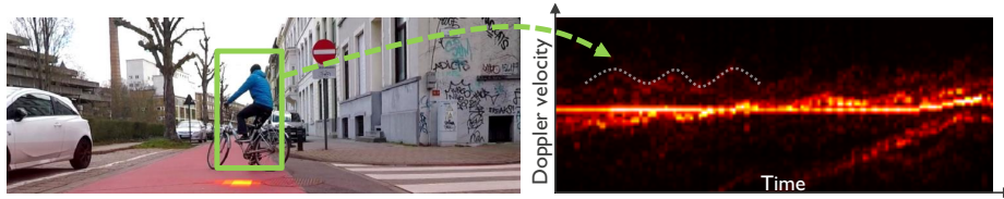
Fig. 1: An example of micro-Doppler patterns. left: The radar signal is projected and overlaid with the synchronized camera image. right: The radar Doppler signal is plotted over time. The micro-Doppler pattern of the cyclist is highlighted by a dotted line.
