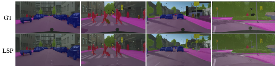
Fig. 2: Qualitative result of segmentation masks on Cityscapes val set. First row shows ground truth mask and second row shows the predicted masks from pruned model.
