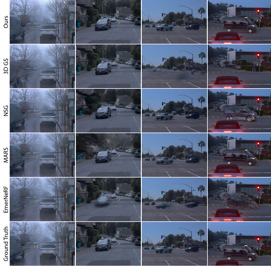
Fig. 4: Qualitative comparisons results on the Waymo [47] dataset. NSG [37] and MARS [60] often produce blurry and distorted results. 3D GS [19] and EmerNeRF [65] generates ghosting artifacts in regions with moving objects. In contrast, our approach significantly outperforms other methods with high fidelity and sharp details.
