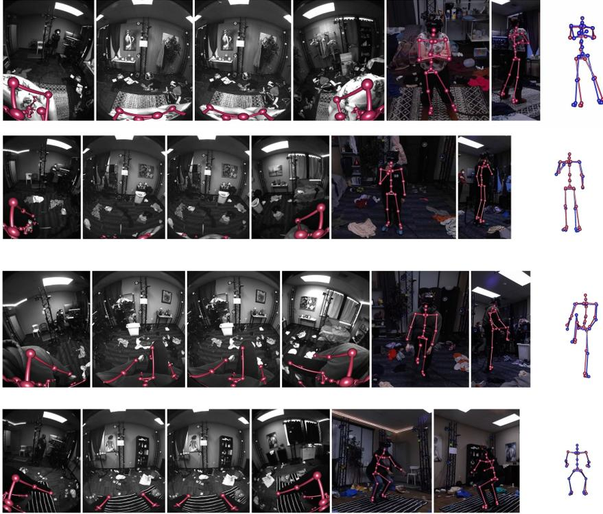
**Fig. 9:** Our model is capable of accurate tracking even in challenging cases, such as (a) arms crossed and out-of-view, (b) scratching the chin, (c) kicking and (d) squatting. Blue denotes ground truth and pink denotes model predictions.
