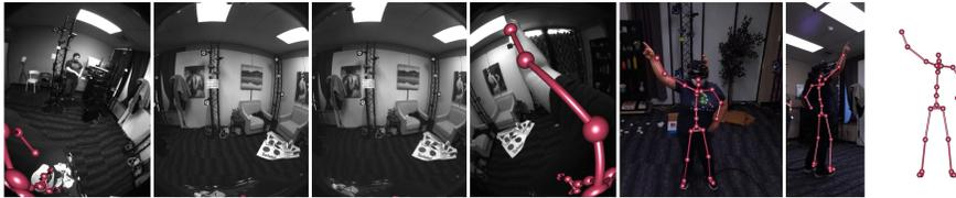
We present the first controller-less egocentric body tracking solution that runs on an actual VR device, using the same four monochrome cameras that are used for SLAM tracking (left). We propose a novel egocentric tracking architecture that models the temporal history of body motion using multi-view latent features, and accurately infers full-body poses even when limbs are out-of-view (right).
