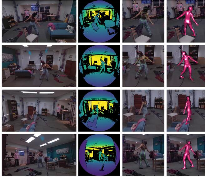
**Fig. 7:** Four of the eight synchronized Azure Kinect images used for ground truth tracking. From left: RGB image, depth image, noisy RGB keypoints, body pose after combined depth and RGB signals. Additional examples can be found in the supplemental materials.
