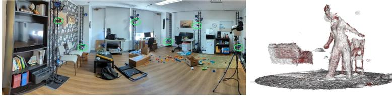
**Fig. 6:** (Left) 6 of the 8 outside-in Kinect cameras are circled in green. (Right) point cloud constructed by fusing depth images from all 8 Azure Kinects.
