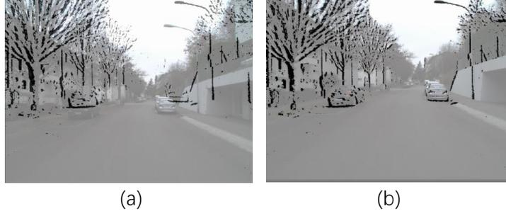
**Fig. 1:** Examples illustrate the comparison before and after the homomorphic transformation. On the left (a): an overlay map of the original RGB image and event image. On the right (b): an overlay map of the RGB image and event image after the homomorphic transformation.
